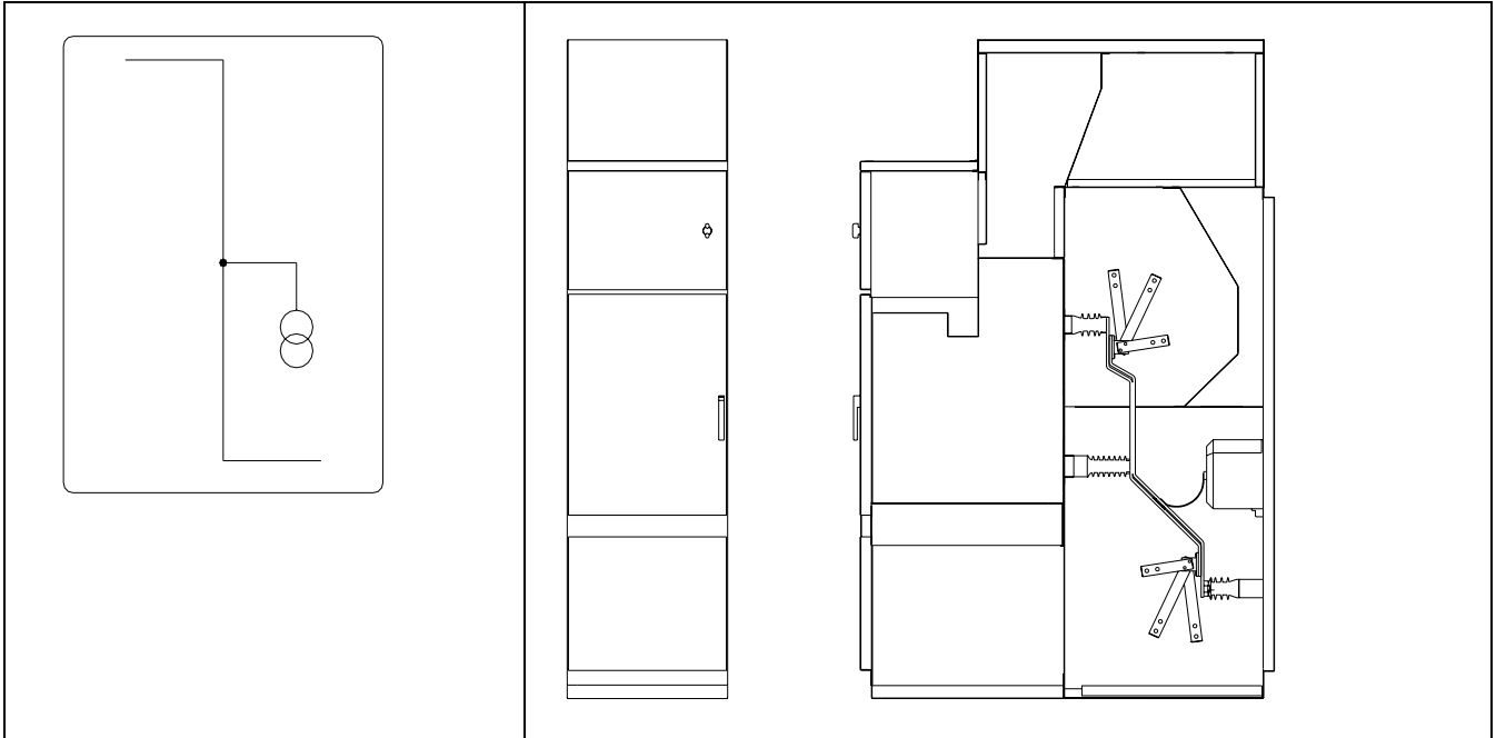
Busbar riser with fixed measuring VT
